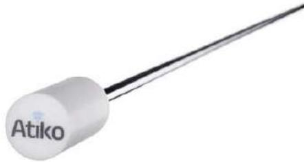
AtikoTI is a device that is used to measure the temperature of liquid, bulk and semi-solid environments using a measuring probe and then transmit this information over a radiolink. The device has an ingress protection of IP63 and works in the temperature range from -40 to +60°C.
